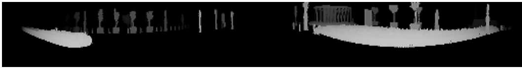
(c) Reference range image projected from the MLS data ( I_{\text{MLS}} )
