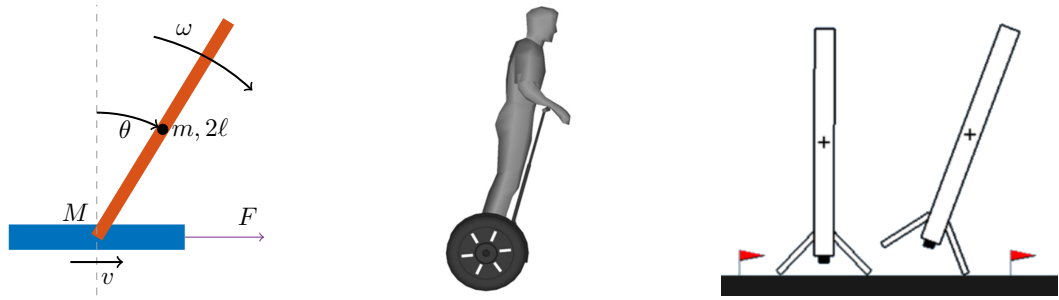
Figure 2.1: A sketch of the inverted pendulum balancing system (left) and the illustration of its potential application in the Segway balancing (middle) and the aircraft landing problem (right). The sources of the middle and right figures are [179] and [180], respectively.
