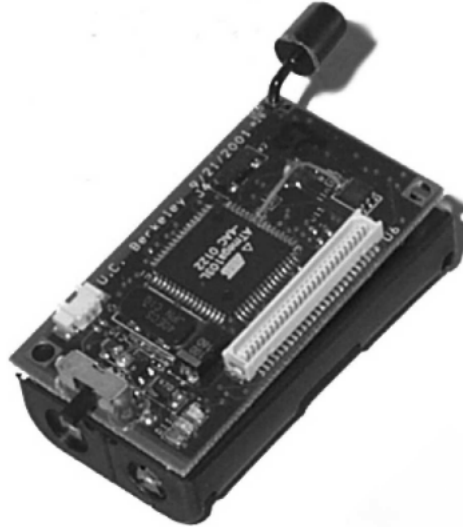
Figure 2.2: The Mica WSN node [25], © 2002 IEEE
