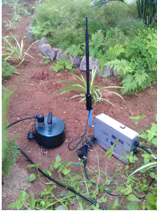
Figure 2.4: Volcano and seismic monitoring with WSN [56]
