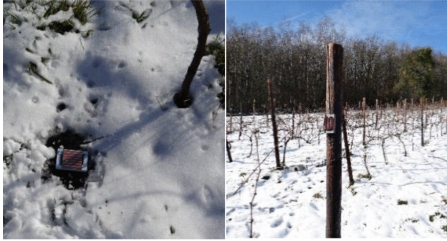
Figure A.4: WSN node with solar EH, deployed in vineyard [224], © 2019 IEEE
