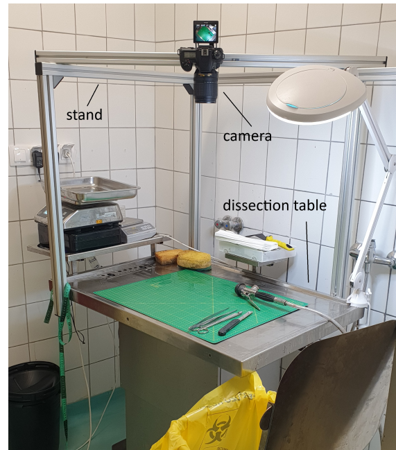
Fig. 1. Setup for macroscopic examination of the placenta and umbilical cord, including a calibrated camera on a stand for later automatization.
