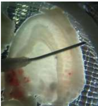
Fig. 1. The inside of the in vitro recording system, where the brain slice is placed on a net that is supplied with artificial cerebrospinal fluid (ACSF), the electrode orientation to the slice (an example). Photo made by N.E.
