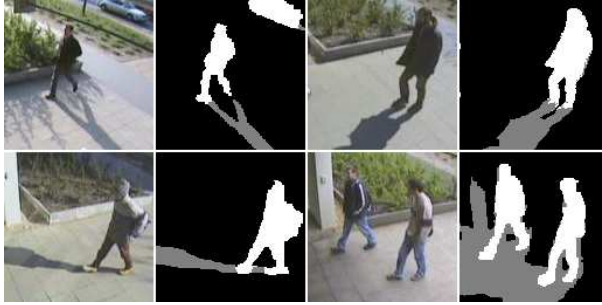
Figure 1: Separation of foreground (white), shadow (gray) and background (black) regions in surveillance videos [Thesis 1].
