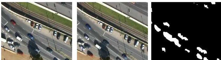
Figure 2: Object motion detection in image pairs captured by moving airborne vehicles. Input images and the resulting mask of independent motions [Thesis 2.1].
