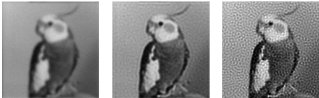
(a) Blurred Image (b) Deconvolved im- (c) Deconvolved im- age after 14 itera- age after 60 itera- tions tions
