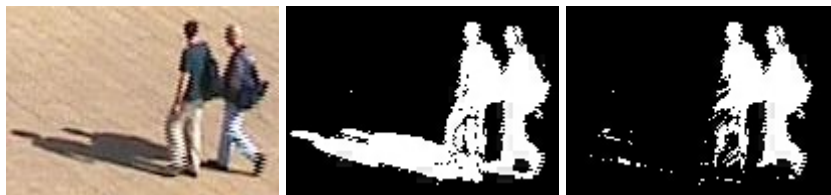
7. ábra: Experimental results on strong shadow. The final foreground mask is the output of the proposed classifier.
