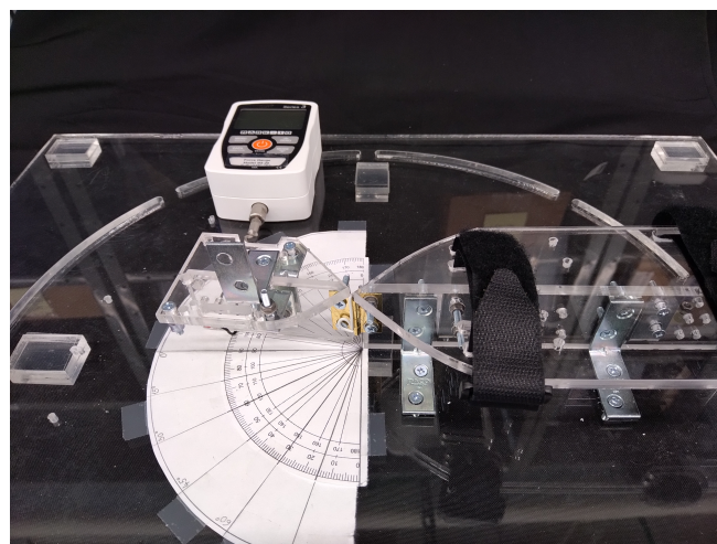
Fig. 1. The torque measurement setup for collecting biological and exosuit assisted wrist torque data. The forearm plate and the hand plate helps to securely fix the position of the lower arm. As the hand plate rotates in a given joint angle by connecting the plate to a force sensor (MARK10 M3-100) positioned perpendicularly to the plate and fixed to the base plate along the circular groove.
