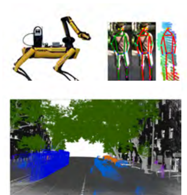
Environment perception from a mobile quadruped robot equipped with LiDAR and camera sensors: results on human pose estimation and 3D scene mapping.
