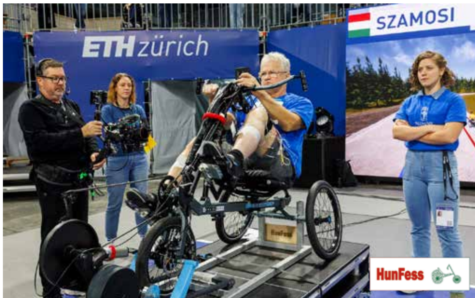
Our pilot on the Cybathlon 2024 FES Bike Race. The tricycle is driven by his paralyzed limbs, a controller sends electrical signals to the selected muscles via surface electrodes to generate muscle forces to drive the tricycle.
