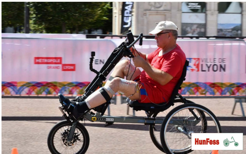
Our pilot on the "Lyon Cyber Days" FES cycling race, as preparation for the Cybathlon FES Bike Race. The tricycle is driven by his paralyzed limbs, a controller sends electrical signals to the selected muscles via surface electrodes to generate muscle forces to drive the tricycle.
