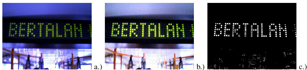
Fig. 2. Color filtering. a.) shows the original picture taken by a mobile phone, b.) shows the color compensated version. On c.) we can see the result of filtering for green-yellow color.
