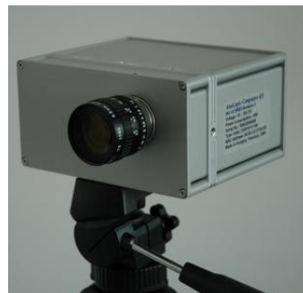
The ACE16K chip, with an 128*128 array of cells, and the Bi-i v2, an extraordinarily high-speed, compact, standalone, intelligent camera, equipped with an ultra fast ACE16K focal-plane array processor.
