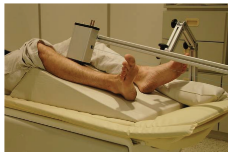
Fig.1. MR-compatible mechanical stimulus presentation equipment
