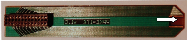
Fig 7. The PCB of the Hungarian acute silicon probe. The white arrow indicates the place to where the back of the silicon electrode will be glued and wire bonded.
