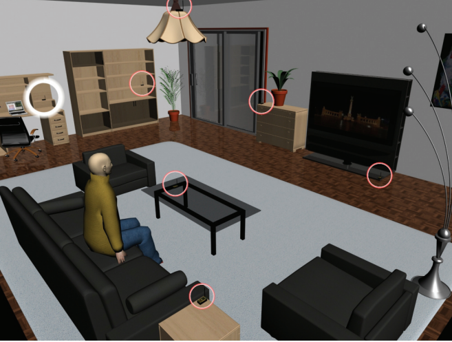
Fig. 1. The room accommodating the patient. The CRUs and the G-CRU installed across the room are highlighted by the thin circles and the thick circle, respectively. The packet transmitted by the implant is received by multiple CRUs, which then cooperatively make the decision on the implant packet. (The illustration was prepared by Dávid Tisza.)
