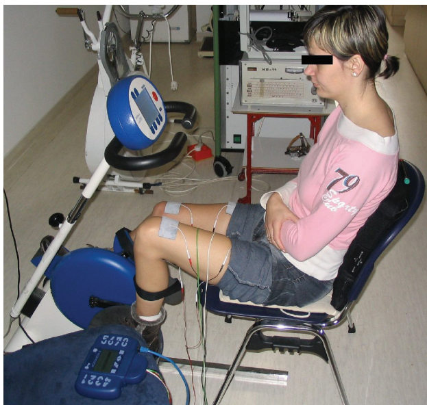
Fig. 3. FES-cycling system. The legs are fastened to the pedals of the ergometer with straps to prevent accidents. The stimulator and some surface electrodes on a SCI patient's muscles are also shown.
