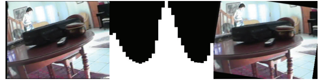
Fig. 3. From left to right: Original frame, edge orientation histogram of the original frame and orientation corrected frame.
