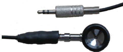
Fig. 2. The bell of the stethoscope for infants
