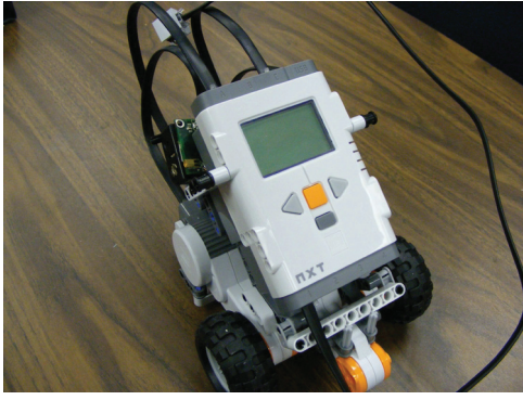
Fig. 1. Mica2 mote mounted on the Lego NXT robot.
