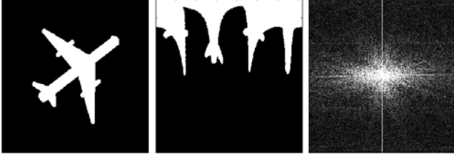
Figure 3: The GFD process: a) The original image, b) the image transformed to polar space, c) the Fourier spectra of the polar image
