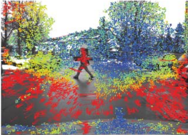
Figure 1. Visualization of considered optical flow fields. Warmer colors encode longer flow vectors.[7]
