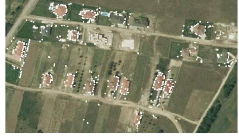
Fig. 5. Enhanced number of Harris keypoints
