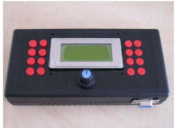
Fig. 2. The stimulator that was developed by Attila Tihanyi and his students. This highly customizable stimulator provides improved functionality in a smaller case compared to the commercially available Motionstim8 stimulator.
