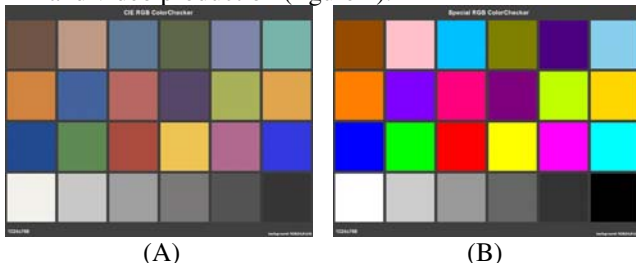
Figure 4. Macbeth Color Checker is a collection of standardized color samples, used for color comparisons and measurements such as in checking the color reproduction of an imaging system or calibrates a device like a digital camera. On the left (A) is the CIE standard, on the right(B) my own Color Chart, based on the original one (A).
