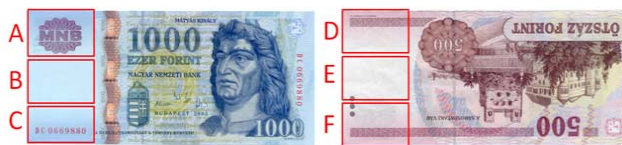
Figure 8. Specific areas for side detection. Three areas (A,B,C) are used during detection, the other three (D,E,F) are just marked to help understanding the method.
