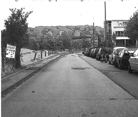
Fig. 2. Canny-edge detection can recognize most of real edges. Combine with graph based segmentation is makes better result. The black lines the result of edge detection
