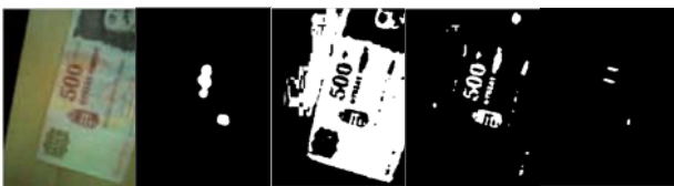
Figure 2. An example for different processing stages. From left to right: input, region of interest, binary image, extracted patterns and extracted holes are shown.
