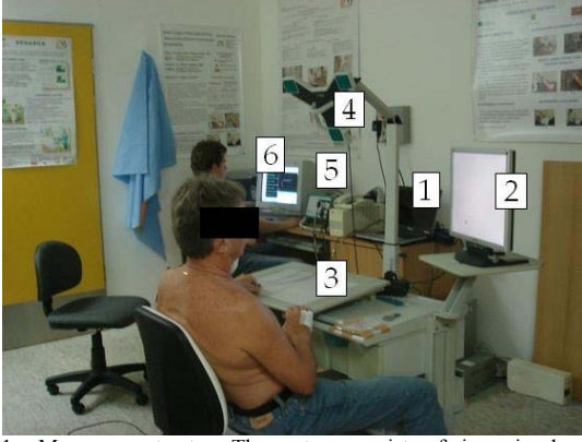
Figure 1. Measurement setup. The system consists of six main elements. 1. Measurement control PC, 2. Stimulus monitor, 3. Digitizer tablet, 4. Movement analyzer ultrasound microphone, 5. Synchronizing hardware element, 6. Movement analyzer control PC
