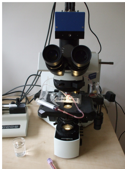
Fig. 1. The constructed biomedical fluid analyzer hydrodynamic focuser with CNN-based camera system. The flow velocity is controlled by precision syringe pump system.
