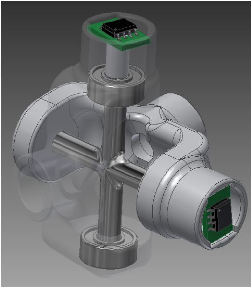
Fig. 3. Two-axis rotational encoder based on rotational hall encoders.
