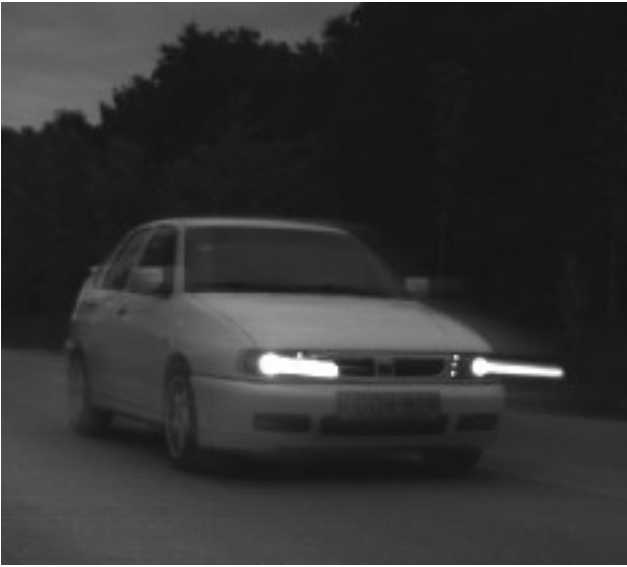
Fig. 2. Superimposed image acquired with the low-GSE Aptina MT9M021 CMOS sensor. The saturated trace represents the movement of the headlights during the readout phase.
