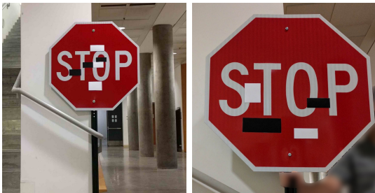
Fig. 2. A sticker based adversarial attack using three dark and three bright stickers on the left ( k = 3 and l = 3 ) and 2-2 stickers on the right ( k = 2 and l = 2 ). These perturbations were tested in real life applications and can cause misclassification in various conditions resulting a threat for the application of convolutional networks. The original image was taken from [6].
