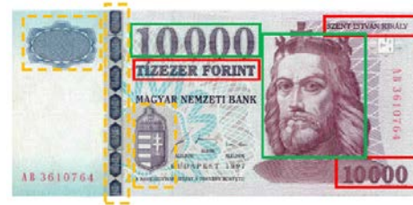
Figure 3. Different components of Hungarian banknotes are shown. Dashed bounding box indicates static objects and continuous the dynamic ones. Static objects appear on each denominations, while dynamic ones change regarding to the actual denomination. Objects within green frames are capable for banknote recognizing tasks, while reds are not due to detection difficulties.
