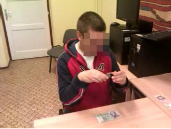
Figure 1. Blind volunteer using the banknote recognition function of the Bionic Eyeglass
