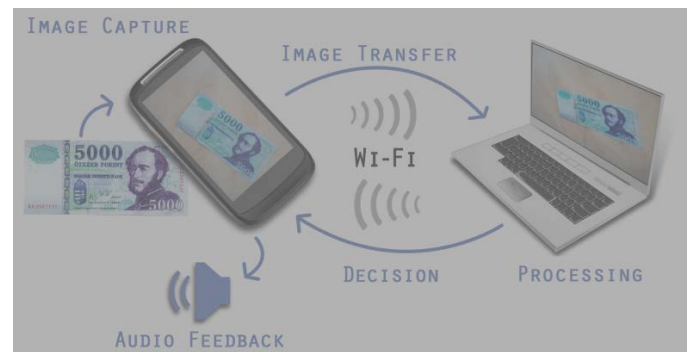
Figure 1. The Bionic Eyeglass prototype – a smartphone interacting with a laptop
