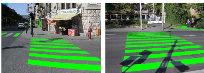
Figure 5. Images show crosswalk patterns detected by the Bionic Eyeglass.
