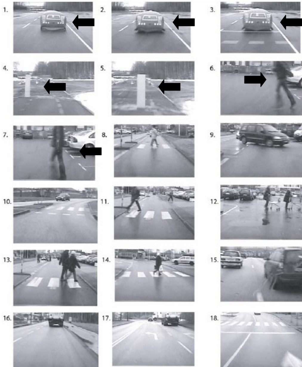
Figure 47 Typical snapshots of test sequences. Black arrows indicate unambiguous collision threats with different objects and persons.
