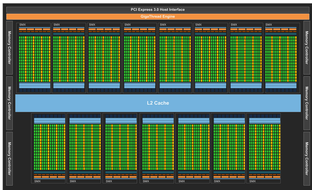
Figure 2.3: A schematic block diagram of the Kepler GK110 chip. Image source: NVidia Kepler Whitepaper [19]. The chip contains 15 Streaming Multiprocessors (SMX). Cache memories, single-precision CUDA cores, and double-precision units are indicated by blue, green, and orange, respectively.
