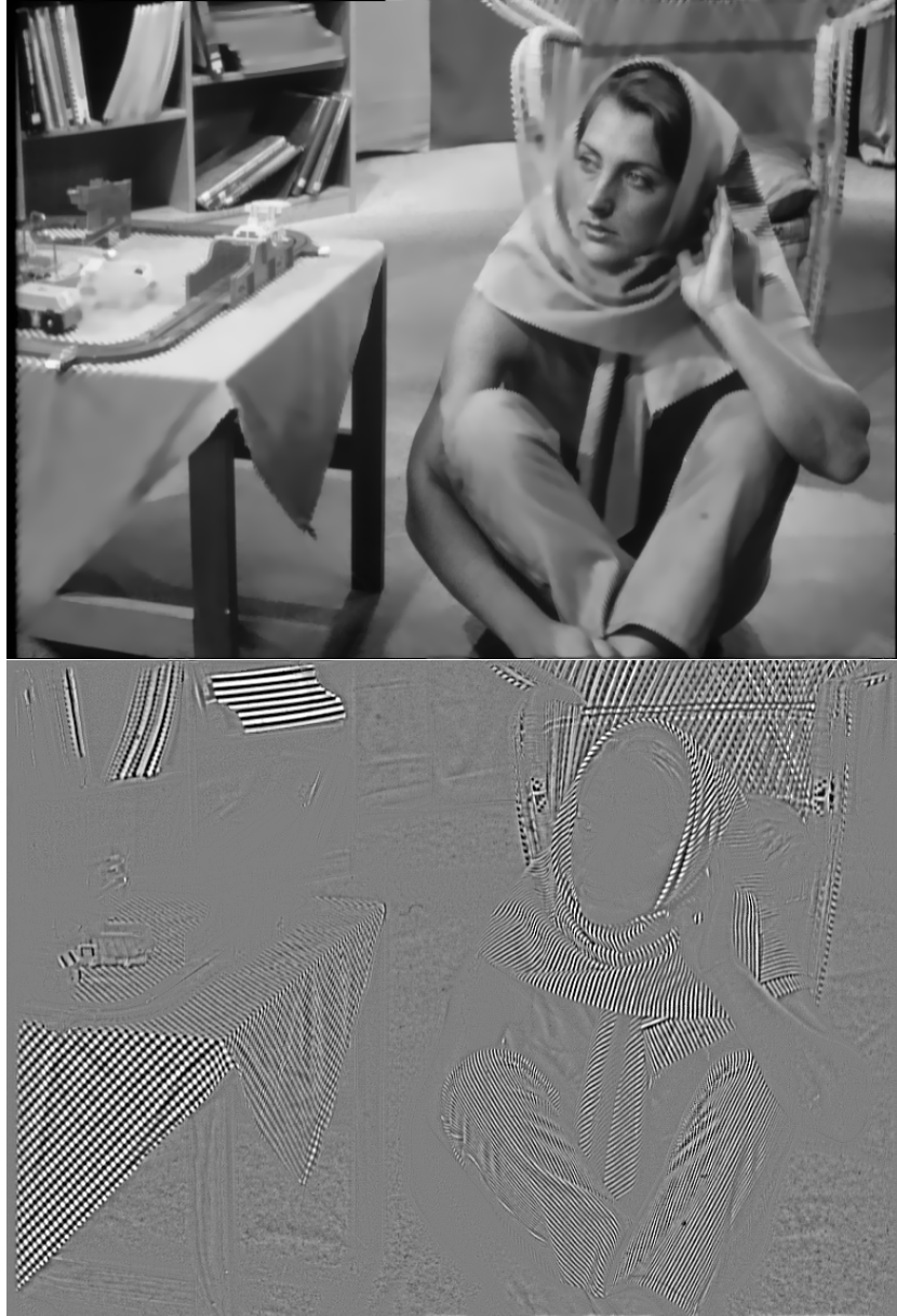
Figure 7.4: The cartoon and texture component of the Barbara image produced by the proposed anisotropic diffusion model with ADE based stopping condition.
