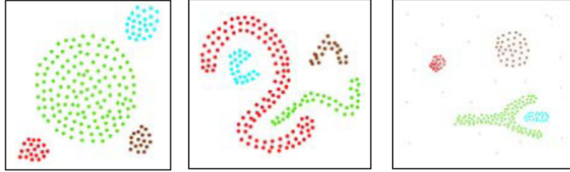
Figure 10.5: Examples of clusters discovered by DBSCAN. Unlike the clusters of k-means, these clusters are not biased to be circular-shaped. [14]
