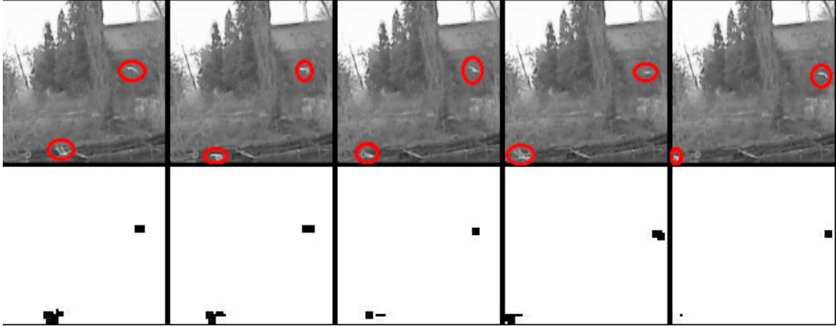
Figure 2.8 Sample consecutive frames from a test video and the corresponding detection maps of the system. The input video shows birds flying in front of a cluttered background (birds are circled in red on the input frames). Since the birds, leaves and branches of the trees are all moving, detecting the targets (birds) is very difficult and must make full use of the capabilities of the multi-channel front-end (such as the ability to filter based on object size and object speed).
