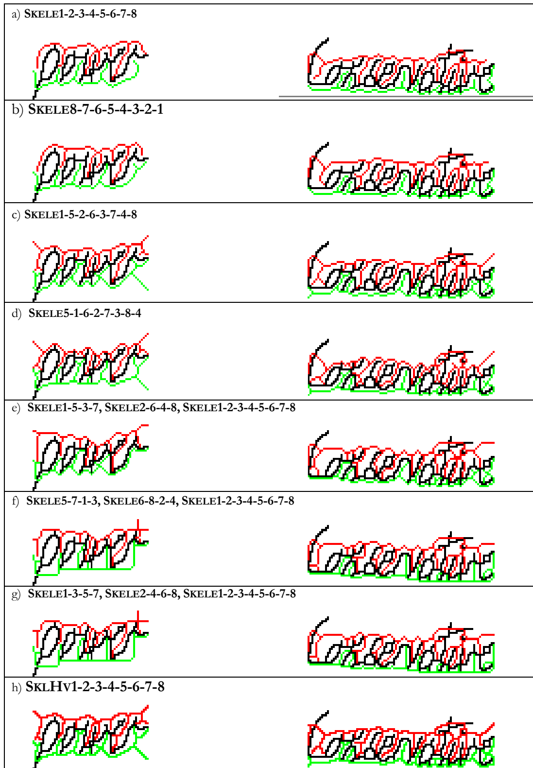
Figure 3.10 Effect of different orderings of the skeletonization on the skeleton. The number sequences after the template base name represent the order of the individual templates used in the iterative skeletonization algorithm (these templates may be found in the Appendix)
