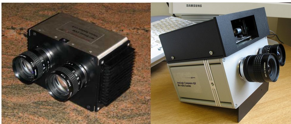
Figure 1.8 The Bi-i Smart Cameras. The left picture shows the Bi-i v1, with 2 sensors, while the right picture shows the Bi-i v2 with 2 sensors and the laser scanner attached
