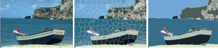
Figure 5. The input (left) is first segmented into clusters that share homogeneous characteristics (center), then clusters that are similar in terms of color and neighborhood consistency are merged (right).
