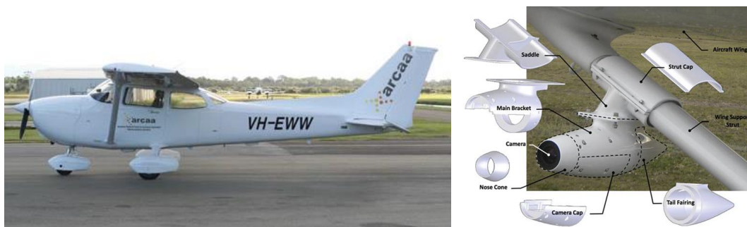
Figure 2.11 Modified Cessna 172 aircraft and the used camera frame
