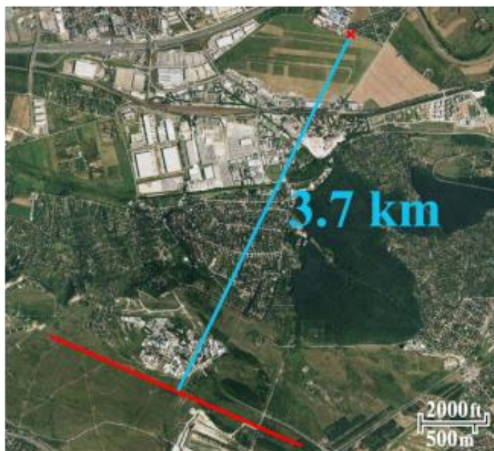
Figure 3.19 Distant aircraft trajectory and camera position; In the image we marked the position of the camera with a red x, the route of the recorded aircraft with a red line, and the distance with blue.
