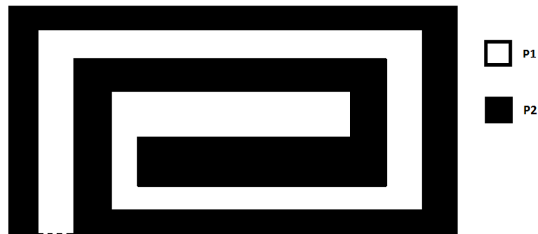
Figure 5.2. 2D example where good bandwidth reduction partitioning leads to unacceptable communication need.
