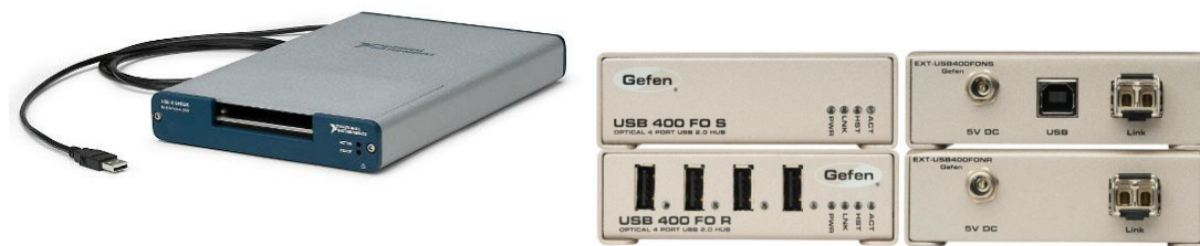
Figure 13. Left NI usb-6353 X series data acquisition device. Right. Gefen USB 400 FO (Gefen, LLC, Chatsworth, CA).
