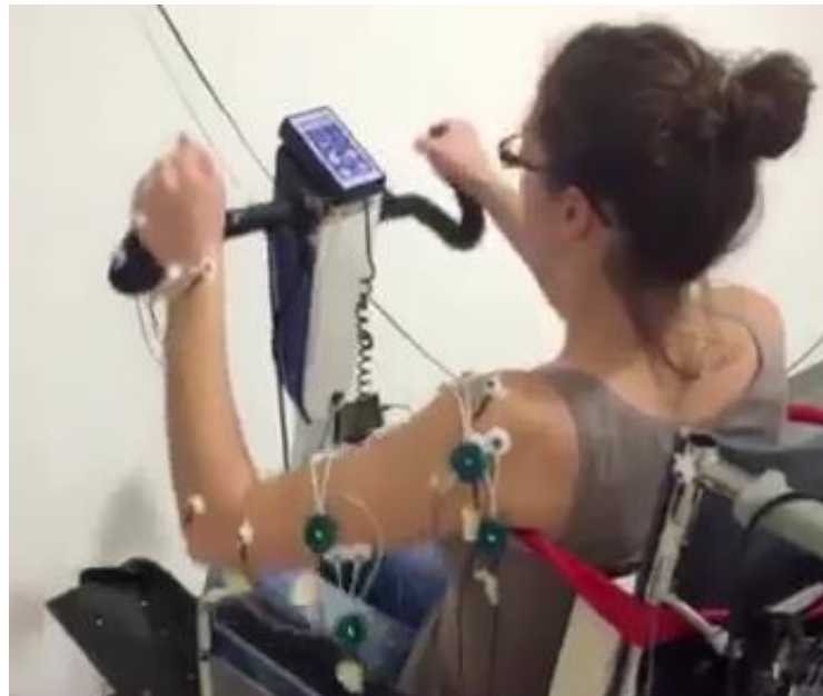
Fig. 1 Cycling arm movements of an able bodied participant while muscle activities (EMG) and kinematic variables are measured.
