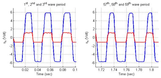
Fig. 1 Case N=16. The metastable periodic rotating wave as shown on the oscilloscope. (Inner state in blue, output in red.) The circuit experiments were made in the bistable parameter region. The oscillation collapses after 74 wave periods and settles down suddenly to an asymptotically stable equilibrium.
