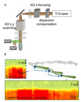
**Fig. 1** A: Block diagram of two-photon 3D Acuosto-optic microscope light path for fast z and lateral scanning. B: Point-by-point continous 3D trajectory scanning of dendritic segments. Examples of Ca<sup>2+</sup> responses: point by point (top left) and continous trajectory
