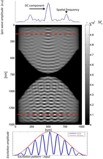
**Fig. 4** A micromagnetic simulation showing the Fourier transform property of a spin-wave lens. The input wave pattern enters at the bottom. The black area is where the B=1.6 T magnetic field is applied. The Fourier transform of the input vector appears as the intensity distribution in the focal plane, at the top of the simulation region.
