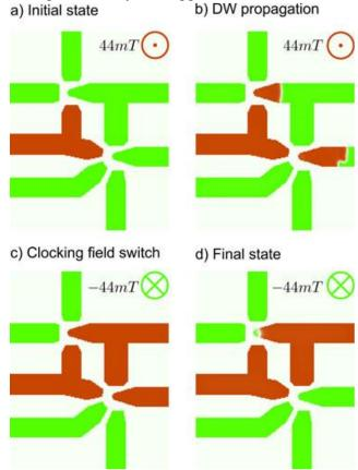
**Fig. 3** Snapshots of a micromagnetic simulation of the threshold gate. The green color represents the -1 state (A, B, -S), red is the +1 state  $(C_{in}, -C_{out})$ . (a) Initial state. (b) DW propagation. (c) Clocking field switch. (d) Final state.
