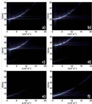
**Fig. 2** Numerically calculated dispersion plots for a YIG-Py bilayer. a) Stand-alone YIG film. b)  $A_{interface} = 0 \text{ J/m c}$ )  $A_{interface} = 0.5 \cdot 10^{12} \text{ J/m d}$ )  $A_{interface} = 1 \cdot 10^{12} \text{ J/m e}$ )  $A_{interface} = 6 \cdot 10^{12} \text{ J/m f}$ ) Single Permalloy film. The YIG mode shifts due to the interaction and an additional Permalloy mode appears
