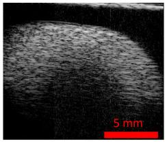
**Fig. 1** Comparison of ultrasound images of an agar-graphite phantom. Left: image taken using commercially available (5 MHz) ultrasound. Right: image taken using high frequency (17 MHz) ultrasound developed by the laboratory. Note the increased resolution at the cost of lower penetration depth. Work with Balázs Bajnok and Marcell Pólik.
