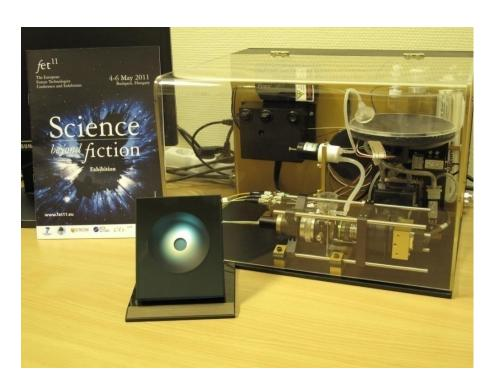
Fig. 2 Multi color digital holographic microscope for monitoring microbiological water quality
