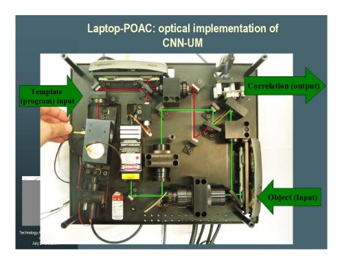
Fig. 1 Laptop-POAC: optical implementation of CNN-UM
