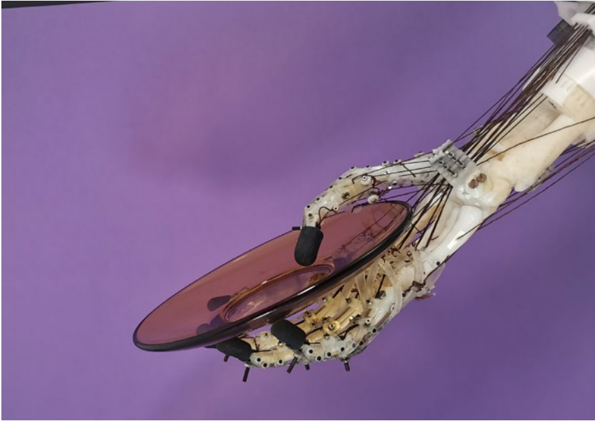
Our anatomically correct hand prosthesis can gently grab delicate objects.
