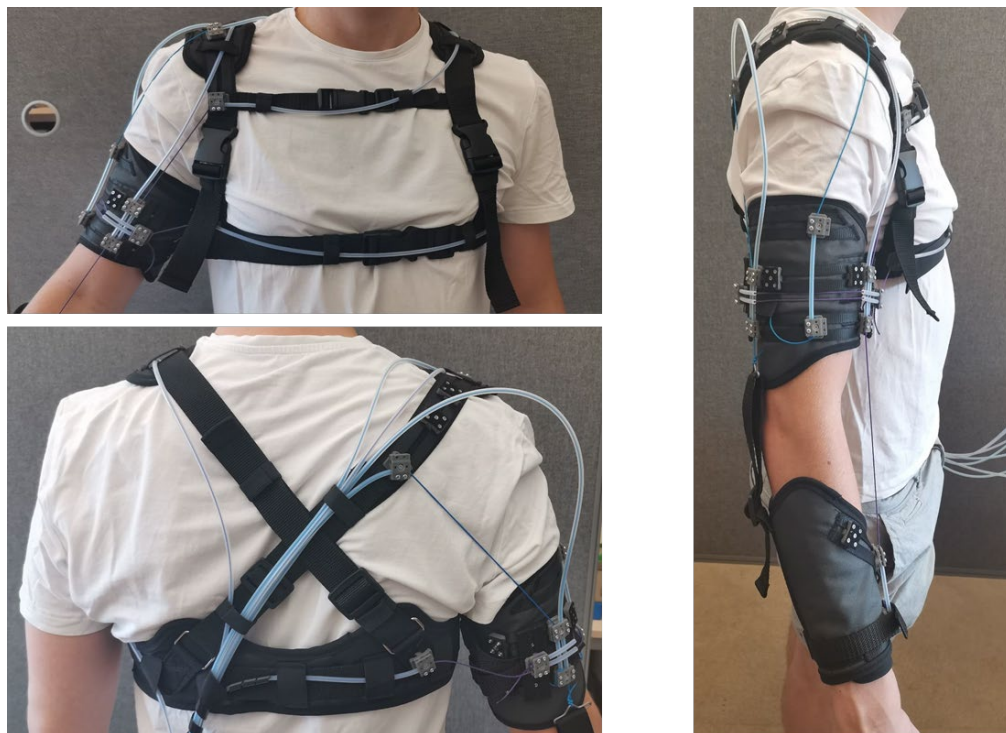
The harness-system (actuating strings, fittings) of the soft exoskeleton prototype.
