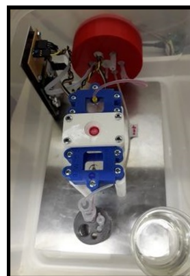
Fig. 1. A measuring system designed to investigate the permeability properties of the artificial skin equivalent [3].
