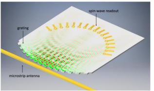
Fig. 1 A schematic drawing of a spin-wave-based spectrum analyzer as described in [1].
