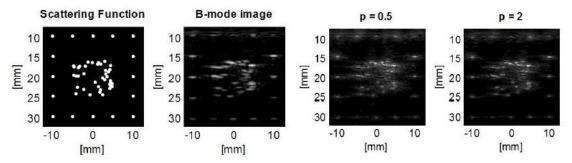
**Fig. 3** 3D Printing methology to test deconvolution algorithms. From left to right: original scattering function design; resulting B-mode image; result of lp deconvolution with p=0.5; result of lp deconvolution with p=2. Image source: [3].
