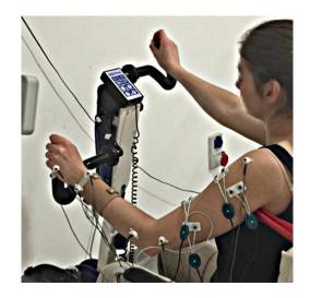
Fig. 1 Arm cranking movements of an able bodied participant. Muscle activities (EMG) and kinematic variables are measured while the participant is arm cranking on an arm-cycle ergometer.
