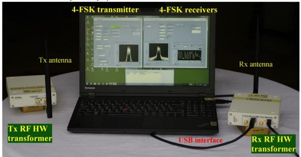
Fig. 2 Universal portable SDE platform testing a 4-FSK radio link.
