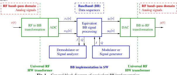
**Fig. 1** General block diagram of equivalent BB implementation.
