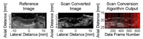
**Fig. 1** Demonstration of scan conversion using manual scanning of a single element transducer. Left: image from reference (commercially available) ultrasound scanner. Middle: demonstration of scan conversion method of same lesion. Right: raw data taken from manual scan, with red lines showing those lines that were selected for scan conversion. Source of image: [7].
