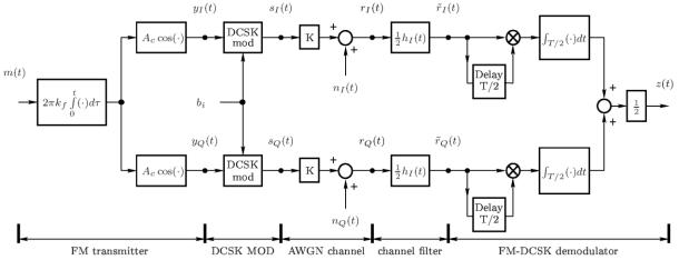
Fig. 3 Baseband equivalent of the FM-DCSK radio link. The BB equivalent of radio channel is also included.
