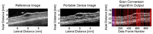
**Fig. 1** Comparison of ultrasound images of a skin lesion. Left: commercial device. Centre: own portable device. Right: scan conversion algorithm in action, with red lines showing scan lines that are selected by our algorithm based on our real-time data-based scan reconstruction algorithm. Image source: [1].
