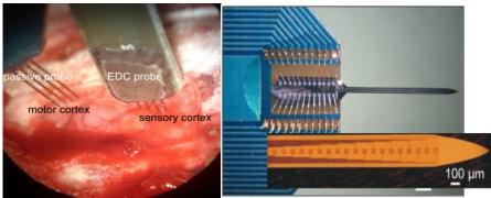
Fig. 1 Brain electrodes with multiple contacts.
