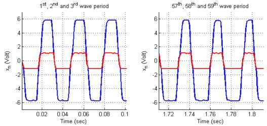
**Fig. 1** Case N=16. The metastable periodic rotating wave as shown on the oscilloscope. (Inner state in blue, output in red.) The oscillation collapses after 74 wave periods and settles down suddenly to an asymptotically stable equilibrium.
