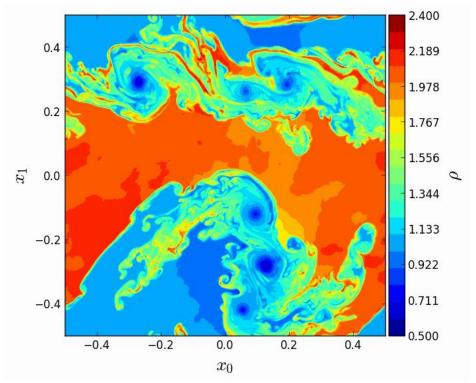
Fig. 1 Kelvin-Helmholtz instability, simulated in OPS. Thanks to the researchers at the University of Southampton for the figure.
