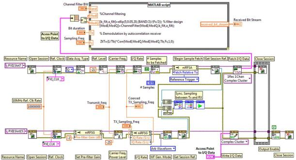
**Fig. 4** Block diagram of the FM-DCSK radio link implemented in SW. The MATLAB script which implements the FM-DCSK receiver is integrated into the LabVIEW environment.
