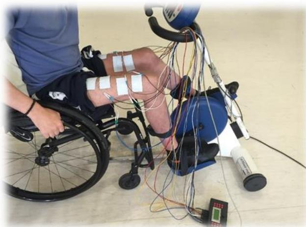
**Fig. 2** Spinal cord injured, lower limb paralyzed patient is cycling on an ergometer in the National Institute for Medical Rehabilitation using a multichannel electrical stimulator device developed at the Pázmány Péter Catholic University.
