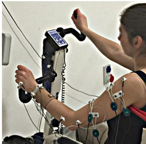
**Fig. 1** *Arm cranking movements of an able bodied participant. Muscle activities (EMG) and kinematic variables are measured while the participant is arm cranking on an arm-cycle ergometer.*
