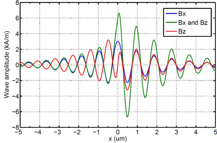
**Fig. 2** Anisotropic spin-wave generation by the microstrip line centered at  $x = 0 \mu\text{m}$  (green), and spin waves generated by applying only the  $x$  (blue) or  $z$  (red) field component of the line.
