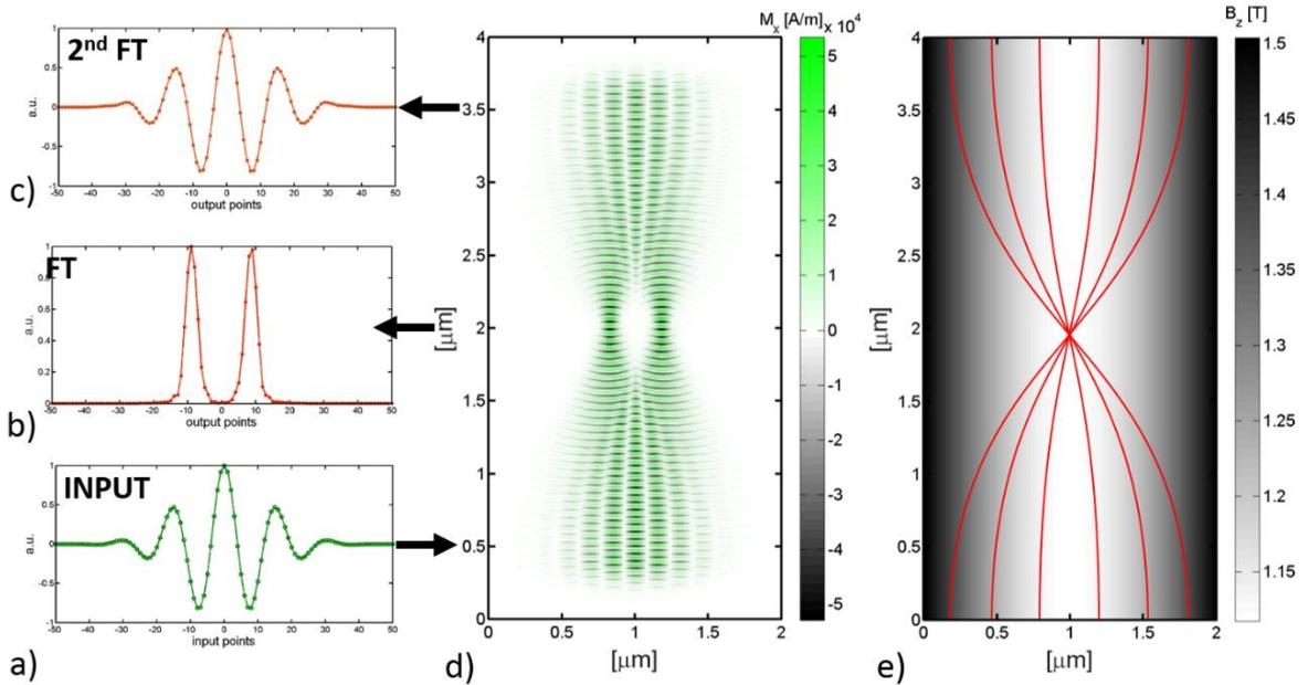
**Fig. 4** Micromagnetic simulation of a GRIN lens performing Fourier transform. a) Morlet wavelet as input. b) Fourier transform performed by the GRIN lens @  $\frac{1}{2}$  pitch length. c)  $2^{nd}$  Fourier transform performed by the GRIN lens @ 1 pitch length. d) Snapshot of the waves propagating in the magnetic film. e) Applied magnetic field distribution to realize GRIN lens.
