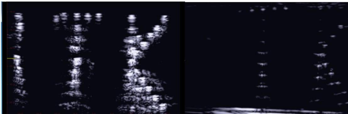
**Fig. 3** Phantoms with the abbreviation of our Faculty, “ITK”. Left: phantom printed with fused filament printing. Right: phantom printed with DLP printing. It can be seen that DLP printing potentially provides higher resolution phantoms, however the lack of the letter “I” underscores the need for ensuring good focussing of the projected pattern. Work with Krisztián Füzési.
