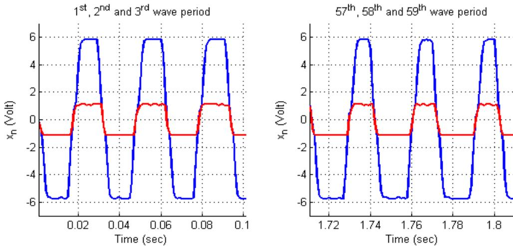
**Fig. 1** Case  $N=16$ . The metastable periodic rotating wave as shown on the oscilloscope. (Inner state in blue, output in red.) The circuit experiments were made in the bistable parameter region. The oscillation collapses after 74 wave periods and settles down suddenly to an asymptotically stable equilibrium.
