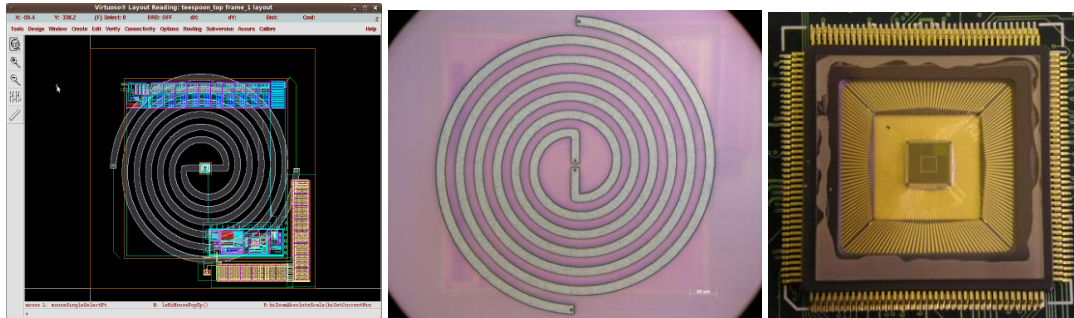
Fig. 2 Different stages of development of a sub-THz imager: design, microphoto, and complete IC.
